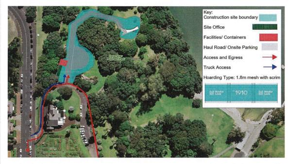
The first stage, scheduled to take 2-3 weeks, will consist of site set-up and include installation of secure fencing around the site and construction of a temporary access road within the park so tools and materials can be brought onsite. This road will be completely removed at the end of the memorial's construction.
